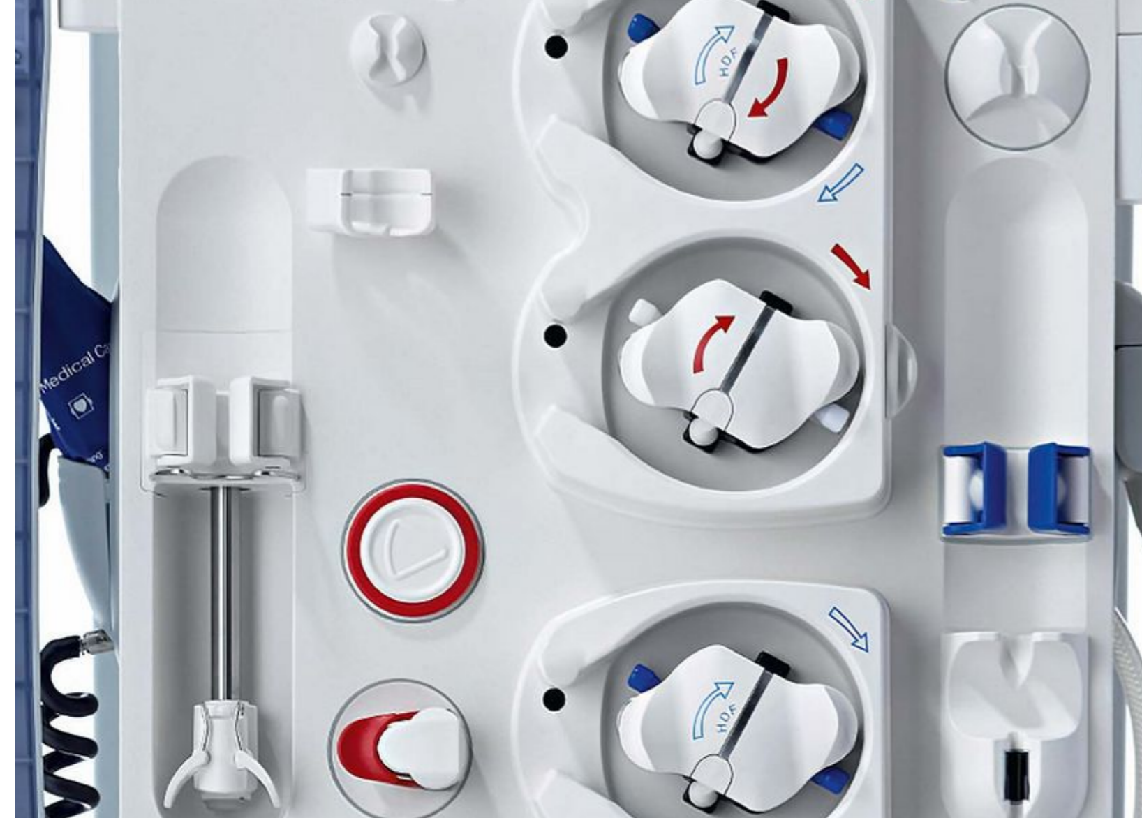
A close up of two substitution pumps that make Mixed HDF possible.
